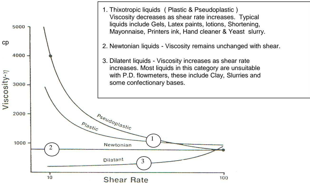
Most empirical and test data for flowmeters and pumps have been developed using Newtonian liquids. When working with Non-Newtonian liquids we use "EFFECTIVE VISCOSITY" to represent the viscous characteristics of the liquid after it has been pre-sheared by the pump. Under these circumstances it is not unusual that the EFFECTIVE VISCOSITY of Thixotropic liquids can be many times less than the theoretical viscosity.
